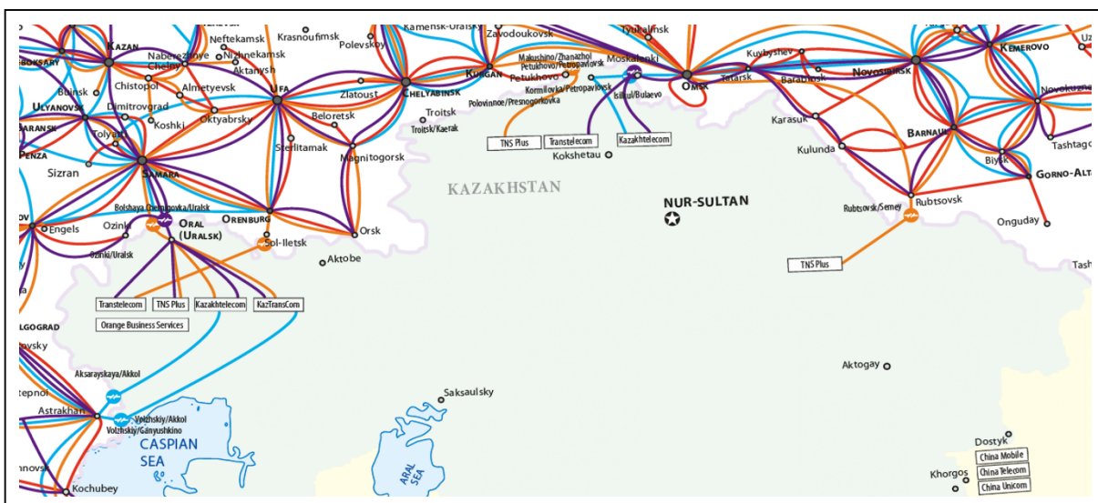
Figure 8: Fibre routes from Russia through the Urals to Kazakhstan, Kyrgyzstan, Tajikistan, and Afghanistan. Traffic transiting these routes crosses Russian networks subject to TSPU and to operator-purchased commercial DPI, exposing neighbouring states to Russian filtering rules. Source: Habr, “Пытаюсь представить жизнь при суверенном интернете в России.” 29
